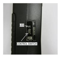
2. Double clicking the **[CONTROL]** switch will toggle through the APCO25 mode (one beep), Voice Inverter mode (two beeps, not available for US consumer model), and CTCSS mode (three
