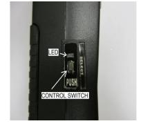
4. To stop recording, press and hold the **[CONTROL]** switch again for <u>two seconds</u>. The red LED will go off.
