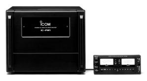
Full-duty 1 kW linear amplifier including an automatic antenna tuner. Has automatic tuning and band selection capability. Full break-in (QSK) operation is possible. The amplifier/power supply unit and the remote control unit are separated.
