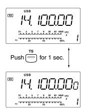
Rotating the tuning dial changes the frequency in 10 Hz steps.
